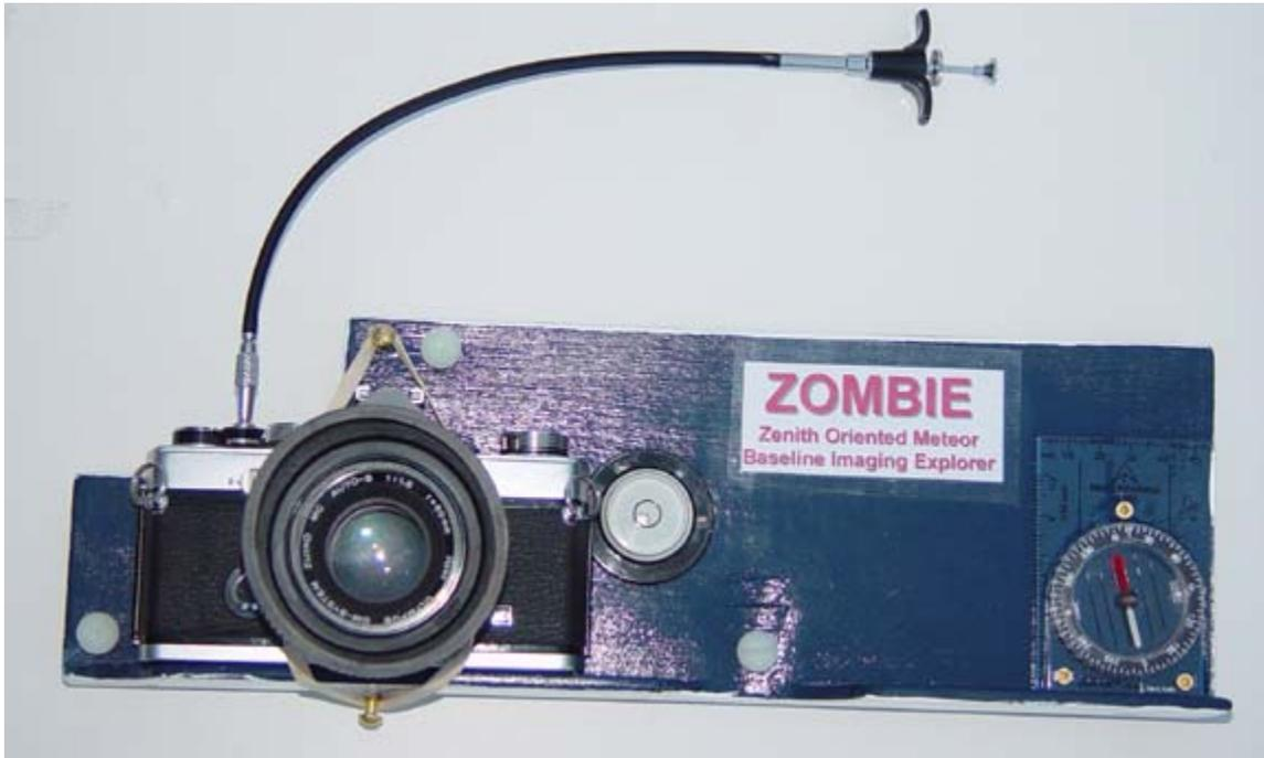
This is a simple and inexpensive camera mount that you can build quickly. It will allow you to quickly and accurately set up the camera and it will produce the standard images we hope to get. But it has no other use than to help you produce images of the zenith that show trailed stars. If you can determine true north and can orient your camera to the zenith you do not need to build this mount.
