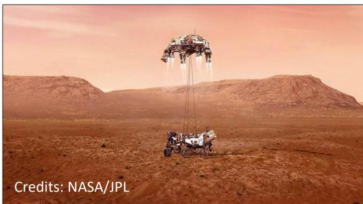
hour (2.7 kph), as it hovers about 66 feet (20 meters) above the surface of Jezero crater. At this point, about 12 seconds before touchdown, the descent stage lowers the Perseverance rover to the surface using a set of 21-foot (6.4 meter) long cables. Once the rover is safely on the ground, the cables are cut and the descent stage flies away for an uncontrolled landing.
