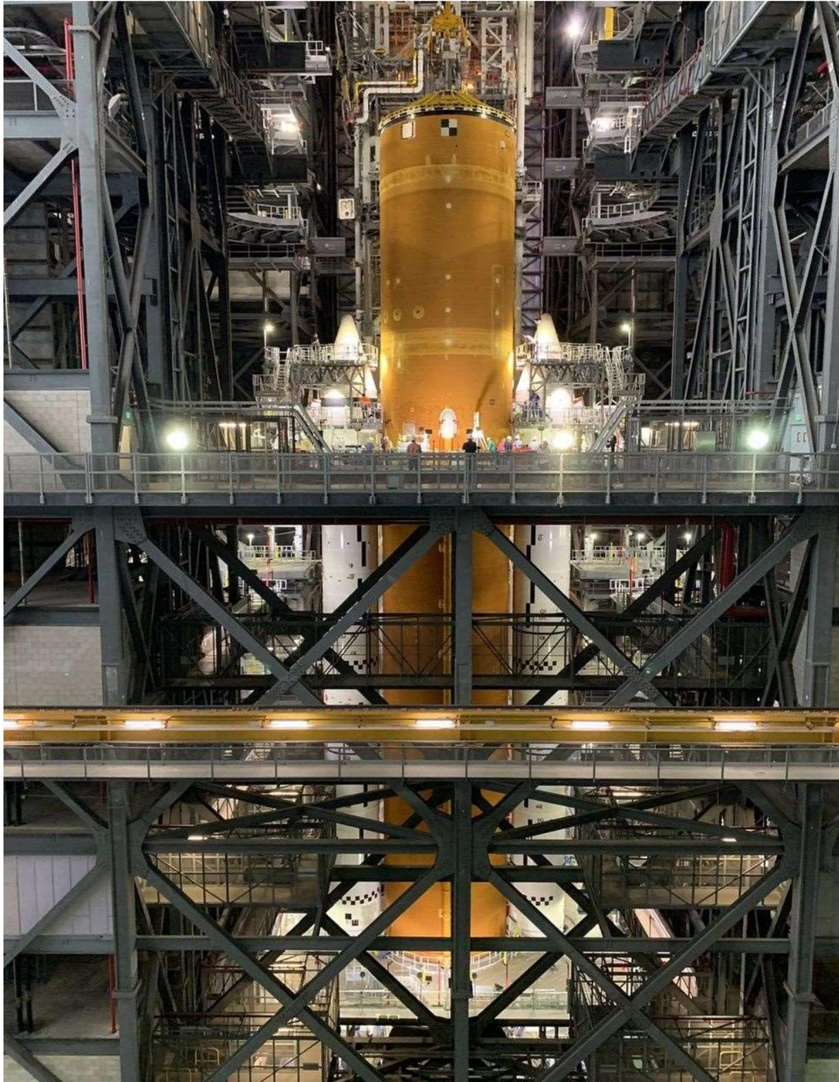
The 212-foot-tall (65 meter) core stage of the SLS seen lowered between two solid rocket boosters for the Artemis-1 launch later this year
