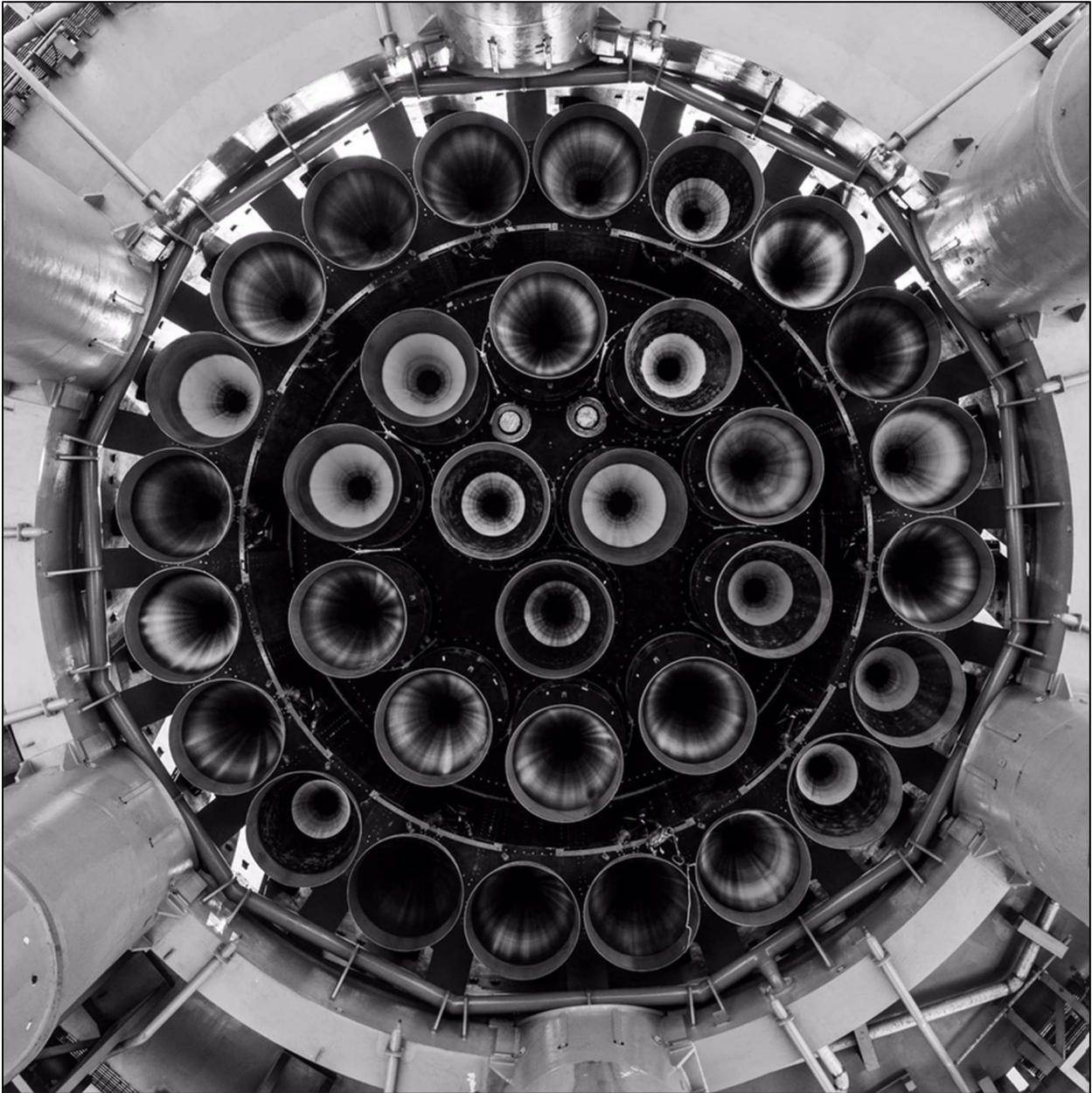
Looking up at the engine compartment of SpaceX's Super Heavy Booster and its 33 Raptor 2 methane-powered engines. The booster underwent a critical all-engine test-firing at Starbase in Boca Chica, Texas, on February 9<sup>th</sup> in preparation for its first orbital flight. Photos of the test-firing can be found on page 11.
