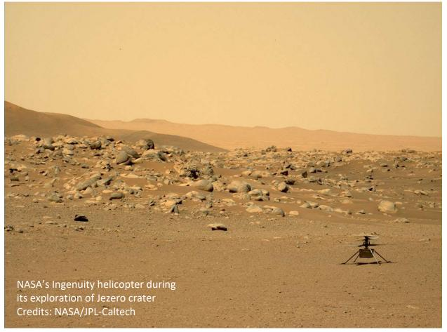
The Mars helicopter was a technology demonstration. Nicknamed "Ingenuity," it rode to the Red Planet attached to the underside of the Perseverance rover, which landed on Mars on February 18, 2021. The little rotorcraft first flew on April  $19^{\text{th}}$  – a 39 second flight that achieved an altitude of about 10 feet or 3 meters. Designed for up to five flights within the 30-day test period, Ingenuity's
