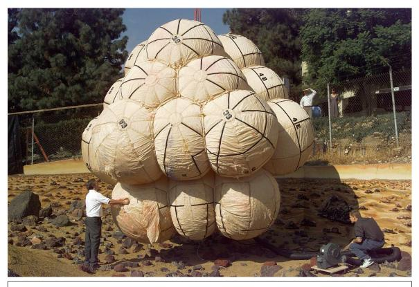
The landing of the Mars Exploration Rovers was cushioned with a cluster of doublebladder airbags (with the rover cradled inside) which were released about 40 - 60 feet (15 – 20 meters above the surface. Credit: NASA/JPL-Caltech
