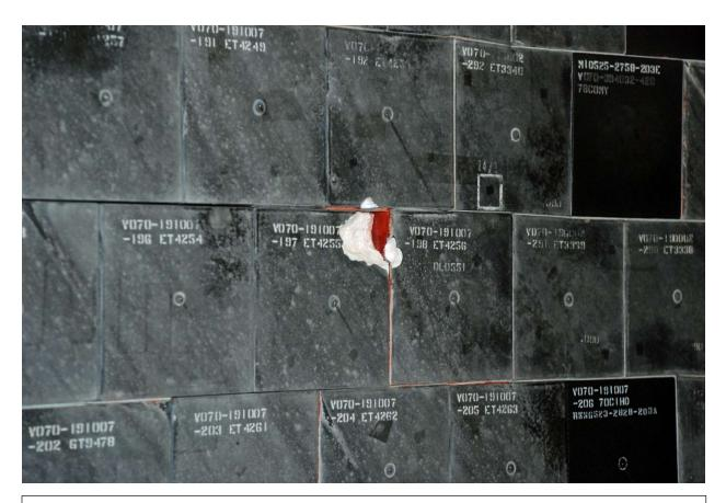
Closeup view of the black HRSI (high-temperature reusable surface insulation) tiles that provided passive thermal control in orbit and shielded the shuttle from the searing heat of reentry when temperatures reached 1,200 -2,300°F (650 - 1,260°C). Damage incurred during its last flight is also visible in a number of the 23,000 HRSI tiles on the vehicle. Photo: Bill Cloutier
