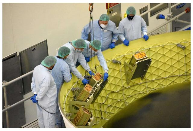
Technicians installing the last of 10 CubeSats in the Space Launch System (SLS) rocket's Orion stage adapter for the Artemis 1 flight in November 2022. Credit: NASA
