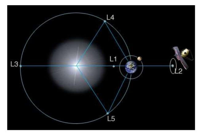
Five locations discovered by mathematician Joseph Lagrange where the gravitational forces of the Sun and Earth (or other large body) and the orbital motion of the spacecraft are balanced, allowing the spacecraft to hover or orbit around the point with minimal expenditure of energy. The L2 point (location of the Euclide and James Webb telescope) is situated 1.5 million kilometers beyond the Earth (as viewed from the Sun).
