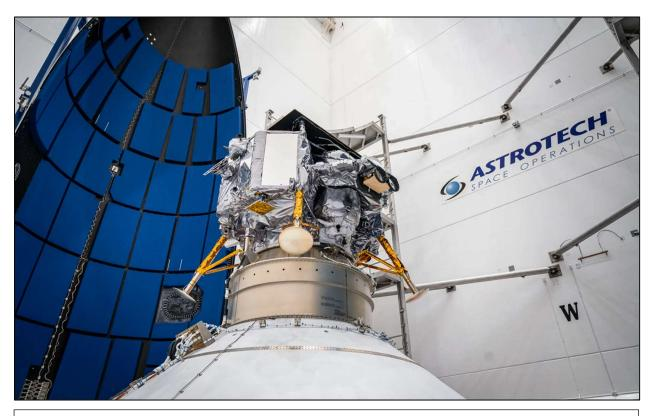
Pre-launch photo of Astrobotic's Peregrine lunar lander prior to being encased within the payload fairings (nose cone) of ULA's Vulcan rocket Credit: ULA
