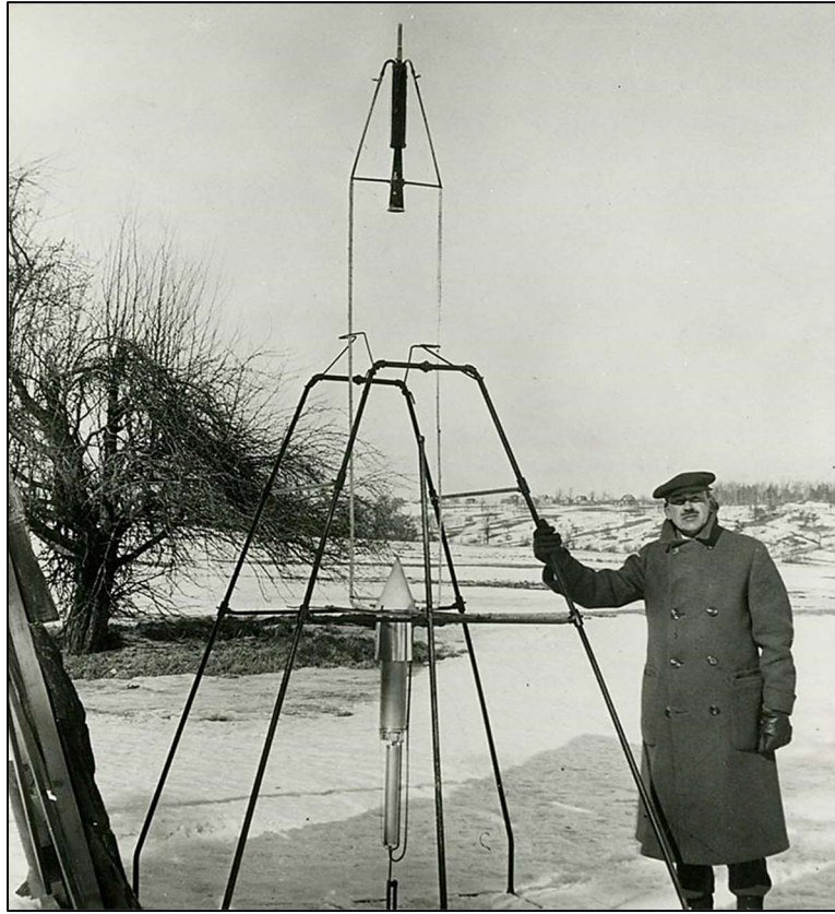
Dr. Goddard with his liquid oxygen-gasoline rocket "Nell" in its launching frame on his aunt's farm in Auburn, MA NASA photo
