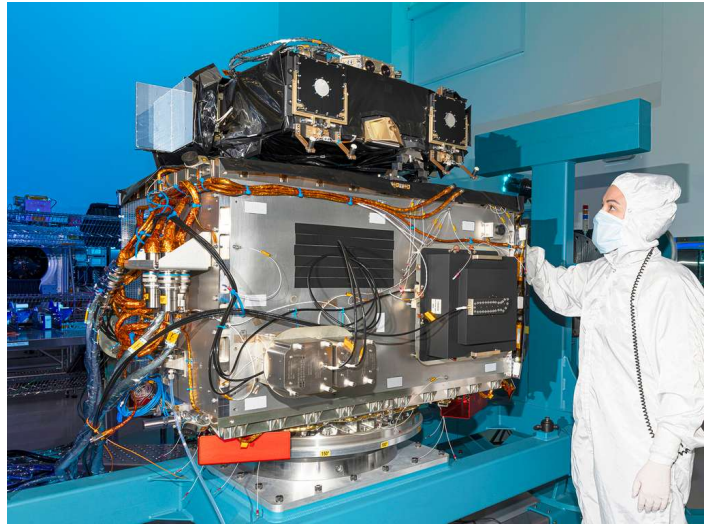
A BAE Systems technician inspects the Carruthers Geocorona Observatory satellite after the integration of the ultraviolet (UV) spectrometer onto the satellite bus.
