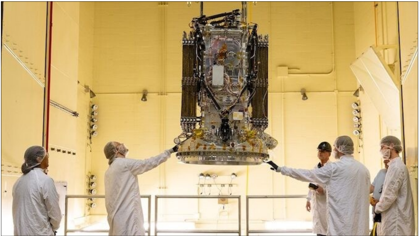
The LINK robotic spacecraft being readied for thermal vacuum testing at NASA's Goddard Space Flight Center in Greenbelt, Md.
