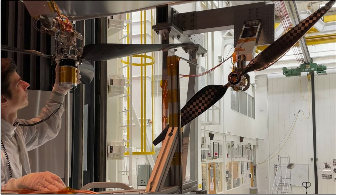
A next-generation Mars helicopter rotor blade prior to testing at supersonic speeds at NASA's Jet Propulsion Laboratory.
