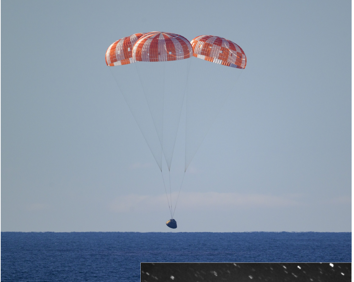
Above: The Orion capsule descending to an ocean landing under its three orange and white main chutes
