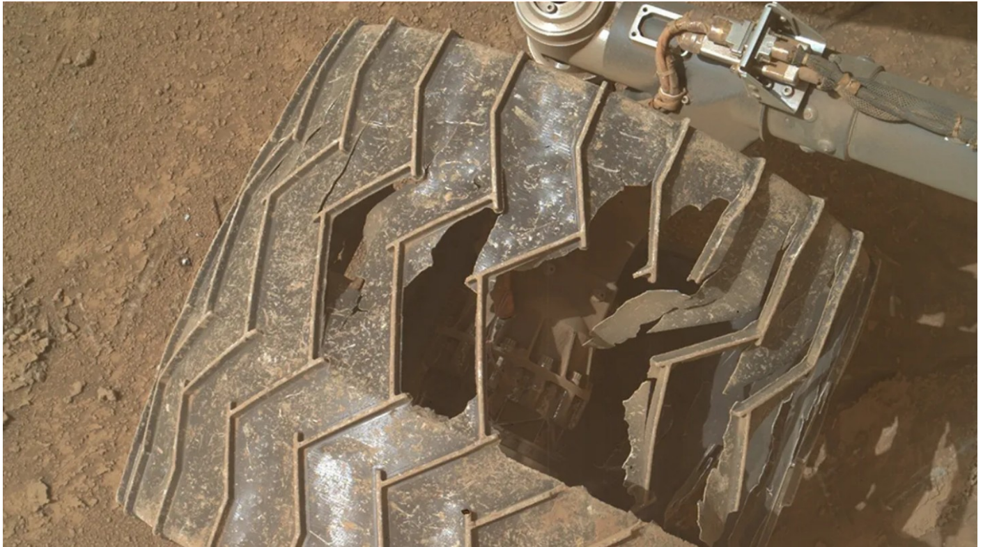
Damaged wheel on the Curiosity rover Image credit: NASA/JPL-Caltech/MSSS
