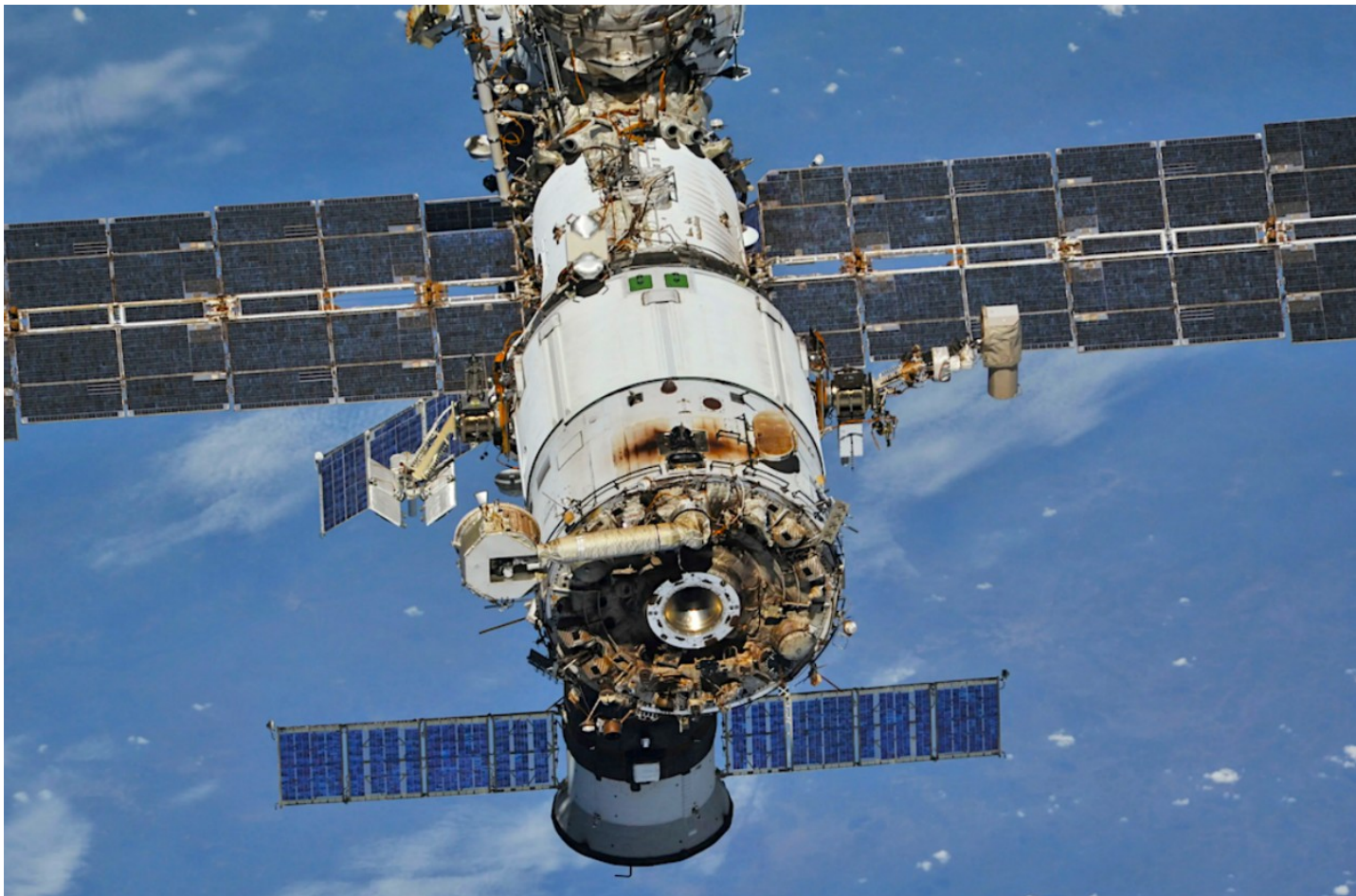
The docking post of the Zvezda module which connects to the leaky transfer tunnel
