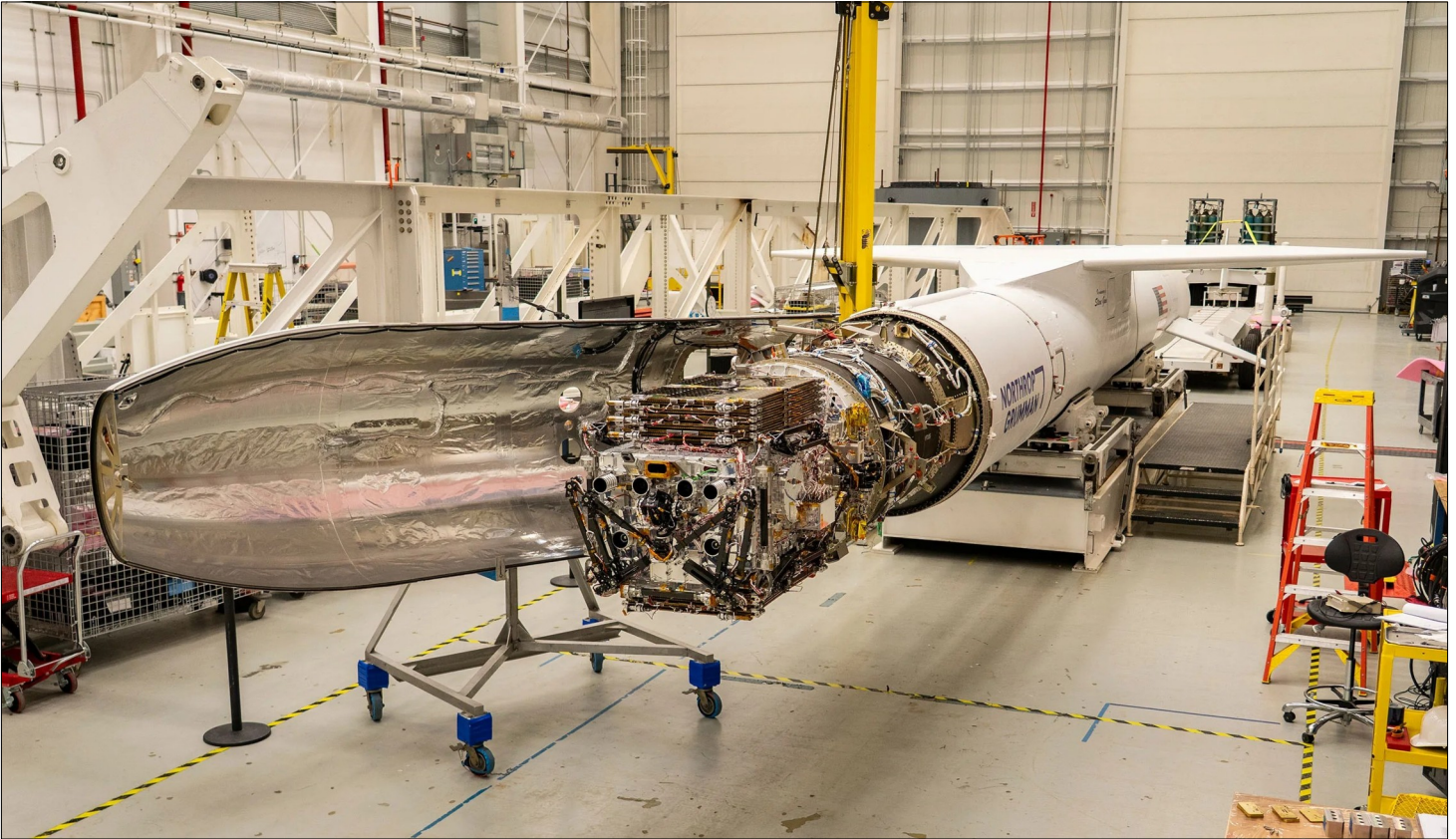
Katalyst Space Technologies' LINK robotic servicing spacecraft loaded aboard a Northrop Grumman Pegasus XL rocket
