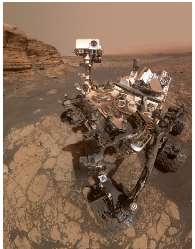
Curiosity rover self portrait combining images from the MAHLI camera on the rover's robotic arm along with images from the Mastcam
