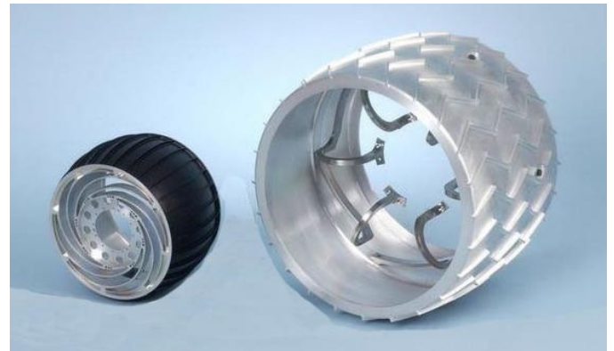
Wheel comparison of the two generations of Mars rovers
