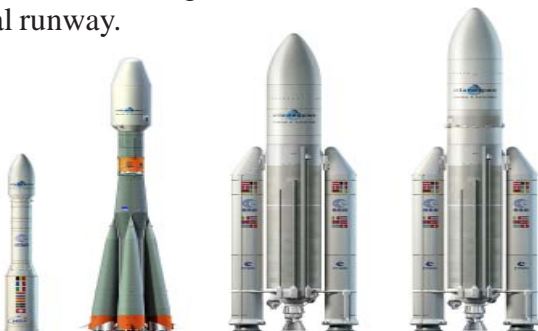
ESA's 'family' of launch vehicles: Vega, Soyuz at CSG, Ariane 5 GS and Ariane 5 ECA .Source: ESA
