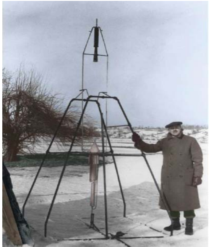
Credit: NASA photo showing Dr. Goddard with his a liquid oxygen-gasoline rocket "Nell" in its launching frame
