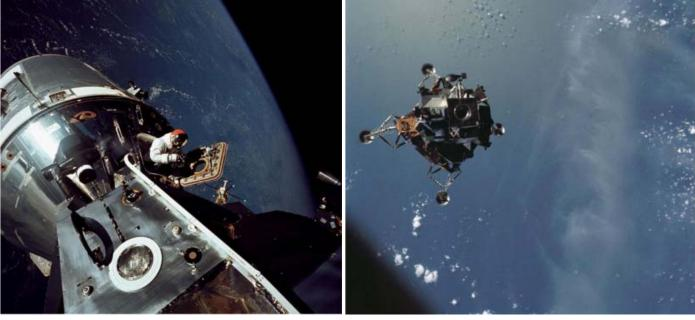
David Scott stands in the open hatch of the Command Module (CM). The photograph was taken by Schweickart on March 6th, from the porch of the LM during his brief excursion outside the vehicle. At that time, the CM nicknamed "Gumdrop" was docked to the LM nicknamed "Spider."
