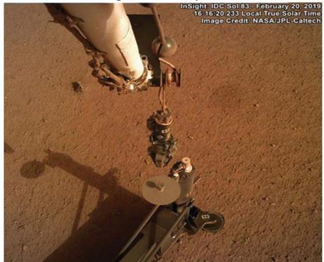
NASA's InSight lander has lowered the Heat and Physical Properties Package (HP3) onto the Martian surface, approximately 3 feet (1 meter) from the seismometer. If all goes according to plan, HP3 will burrow
