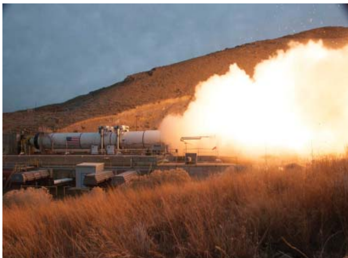
Static firing of the 5 segment solid rocket booster Image Credit: Orbital ATK
