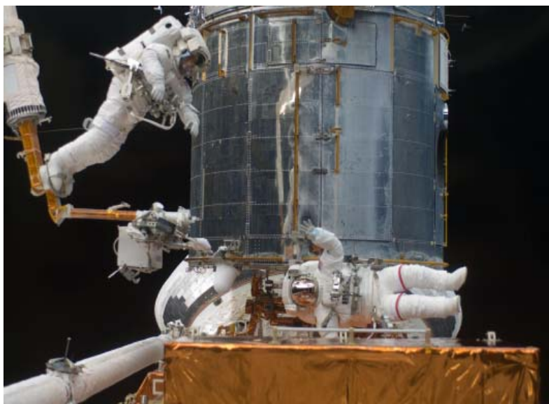
Mission Specialists Andrew Feustel and John Grunsfeld servicing the Hubble Space Telescope on the end of the remote manipulator system arm, controlled from inside Atlantis' crew cabin. Image credit: NASA
