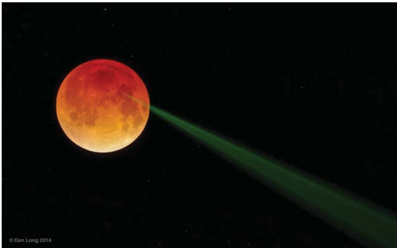
A green laser beam from the Apache Point Observatory targets the reflector at the Apollo 15 landing site during the April 15th total lunar eclipse. Photo credit: Dan Long (Apache Point Observatory)
