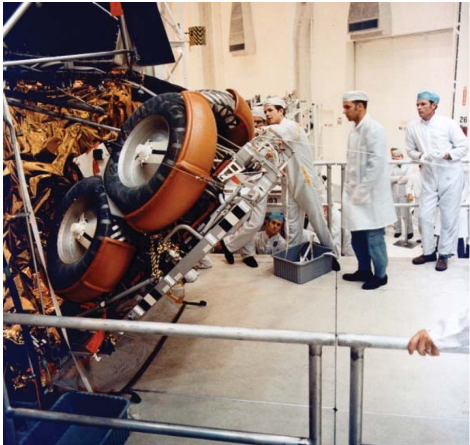
Astronaut David Scott (center) watches as technicians fit check the folded Lunar Roving Vehicle in an exterior bay of the Lunar Module. The rover was deployed by the astronauts once on the Moon's surface using a system of pulleys, ropes and cloth tape. Photo Credit: NASA
