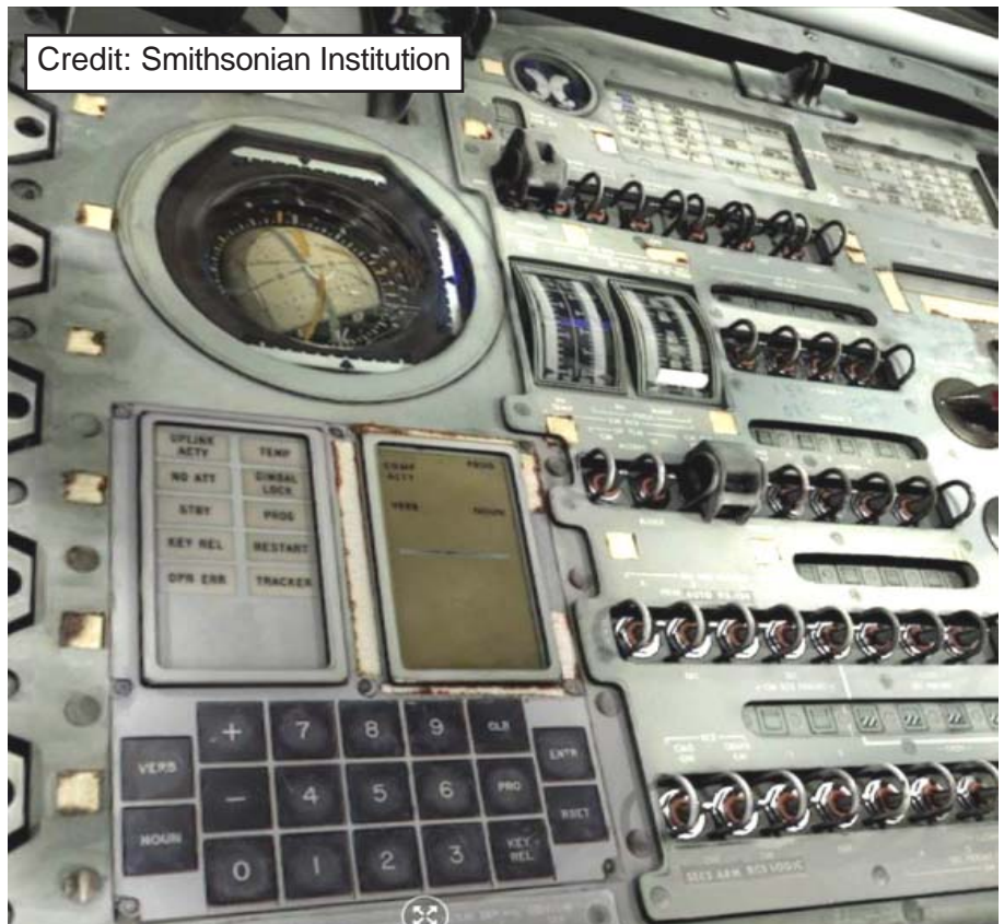
Main console with one of the Flight Director/Attitude Indicators (8-ball) and the Guidance Computer's Display and Keyboard.
