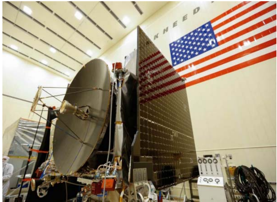
Assembled spacecraft readied for environmental testing Credit: Lockheed Martin Corporation
