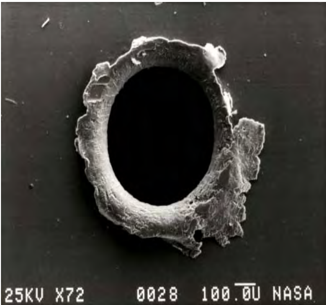
View of an orbital debris hole made in the panel of the Solar Max experiment. Source: NASA Orbital Debris Program
