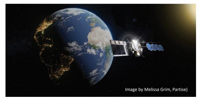
AFRL will customize the bus for the Arachne spacecraft to host the Space Solar Power Radio Frequency Integrated Transmission Experiment or SSPRITE. The demonstration project will assess technologies that convert solar energy to radio frequency power, as well as the feasibility of transmitting and converting that power to a usable form back on Earth.
