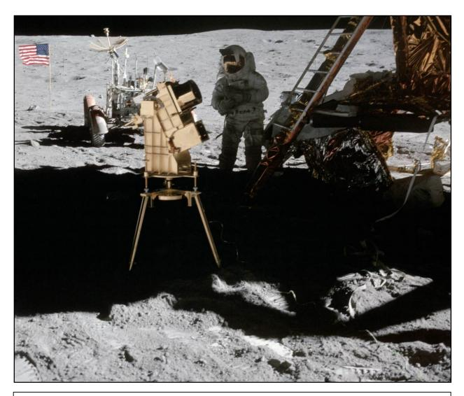
The first camera/spectrograph used to make astronomical observations from the surface of another planetary body - set up by the Apollo 16 astronauts. Credits: NASA
