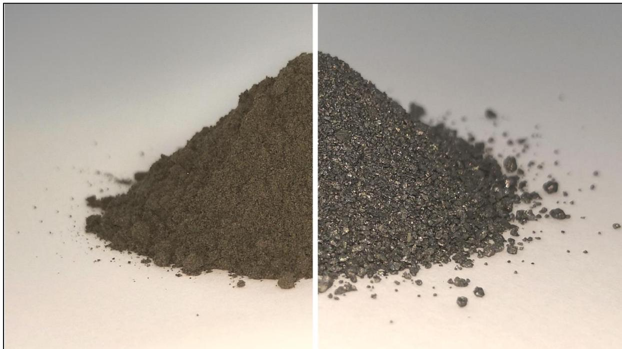
Before and after images of a sample of simulated lunar soil regolith in which essentially all the oxygen has been removed. The end product (right) is a mixture of metallic compounds.
