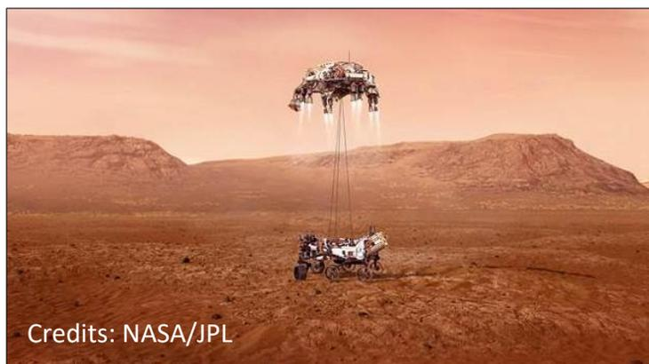
hour (2.7 kph), as it hovers about 66 feet (20 meters) above the surface of Jezero crater. At this point, about 12 seconds before touchdown, the descent stage lowers the Perseverance rover to the surface using a set of 21-foot (6.4 meter) long cables. Once the rover is safely on the ground, the cables are cut and the descent stage flies away for an uncontrolled landing.
