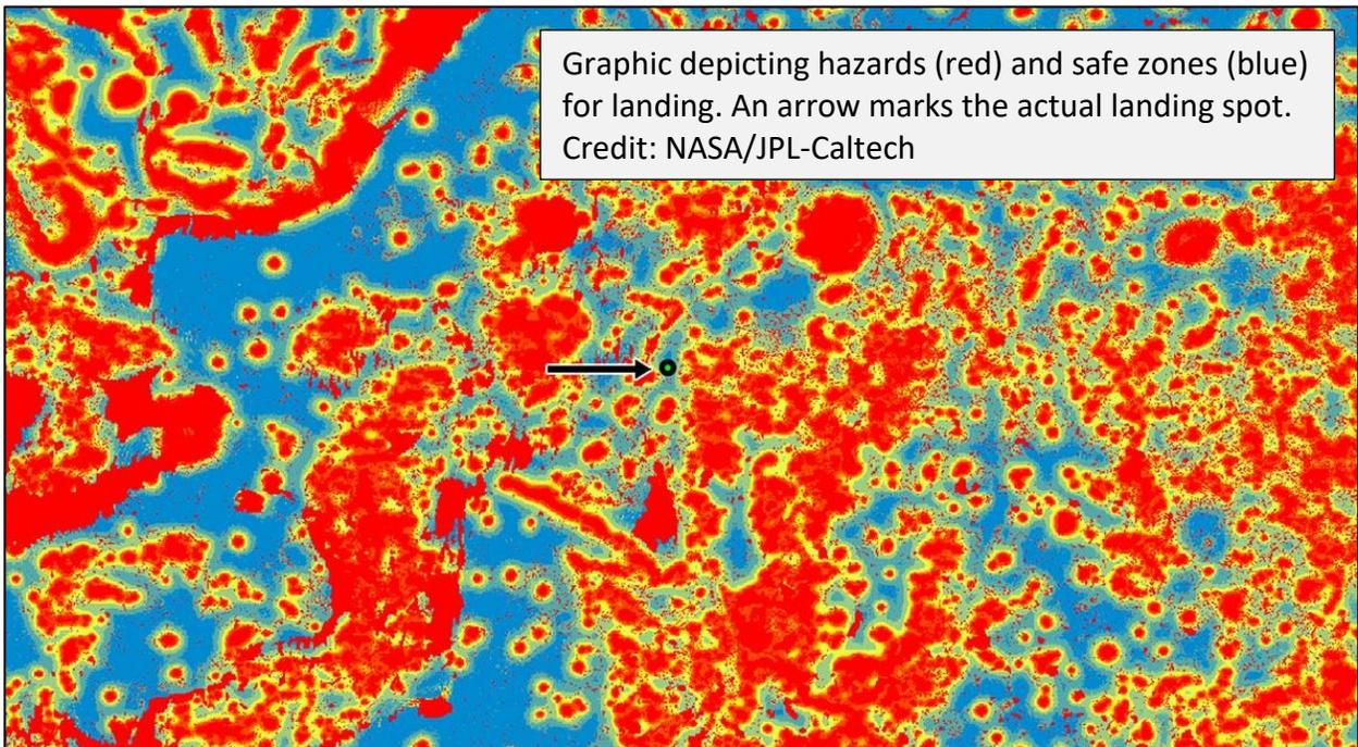
The spacecraft was equipped with two new technologies (Range Trigger and Terrain Relative Navigation) for landing the 2,263-pound (1,026-kg) rover on a hazard-free spot on the crater floor. Perseverance landed about 1.1 miles (1.7 km) from the center of the targeted area. The site is level and free from any large boulders or other obstacles with the rover reporting only a 1.2° tilt.
