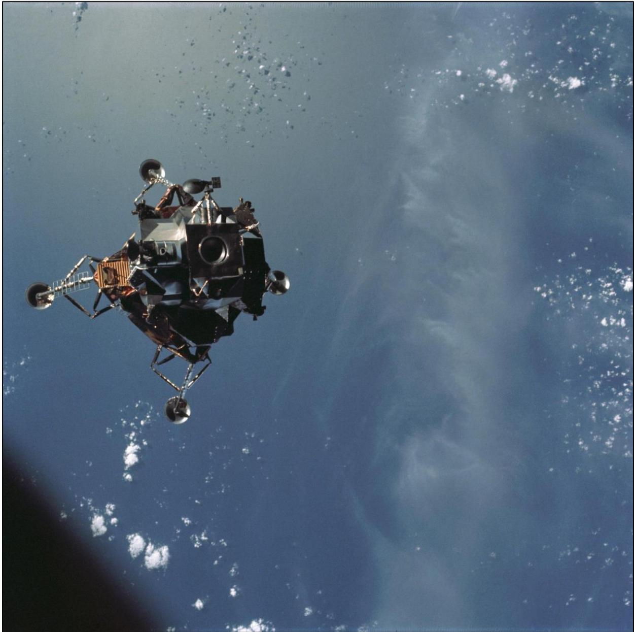
A view of the free flying LM with its landing legs extended captured on March 7<sup>th</sup> by David Scott who remained in the CM while McDivitt and Schweickart checked out the LM. The circular opening in the top of the ascent stage allowed astronauts to transfer between vehicles when docked.
