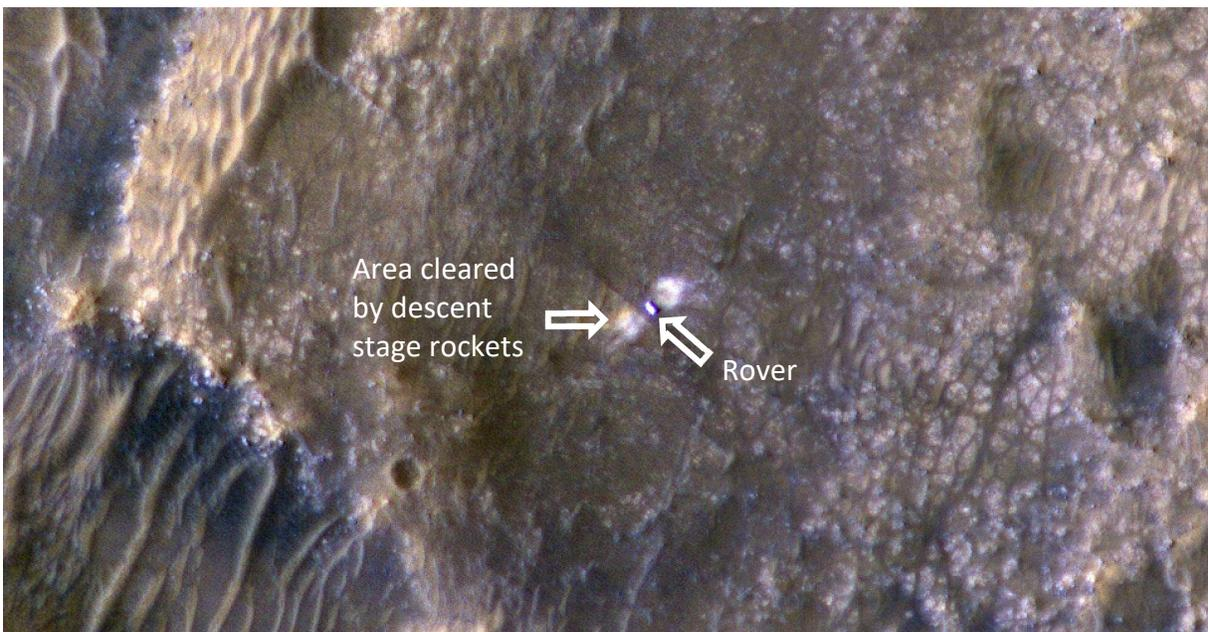
Sixty-one years later, the Mars Reconnaissance Orbiter's camera is able to resolve the 10-foot-long (not including the arm), 9-foot-wide (about 3 meters by 2.7 meters) Perseverance rover from an altitude of 180 miles (290 km). (Image Credit: NASA/JPL-Caltech/University of Arizona)
