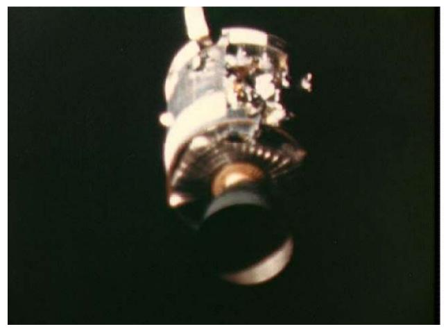
Damaged Apollo 13 Service Module photographed after the Command Module separation Photo: NASA
