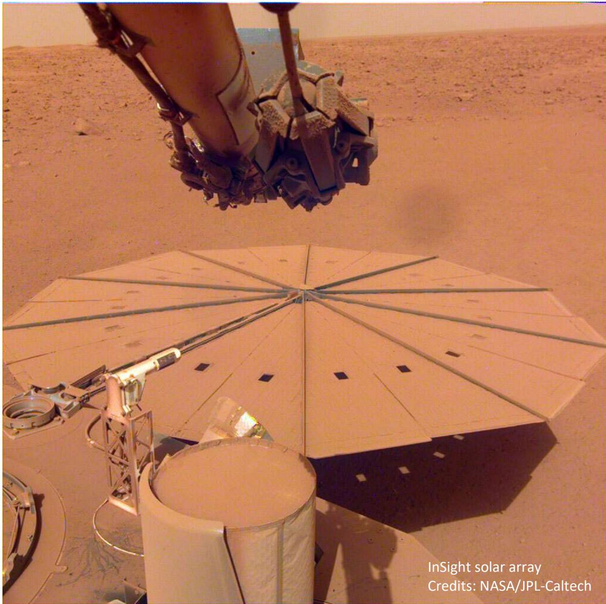
NASA's InSight mission is coming to an end. The lander's dust laden 7 foot wide (2.2 meter) solar panels are now producing 500 watt-hours each sol compared to the 5,000 when they landed in November 2018 (enough to power an electric oven for just 10 minutes today vs. an hour and 40 minutes at landing). Science operations, with winter approaching and the amount of dust in the atmosphere increasing, are becoming more challenging with power levels nearing critical levels.
