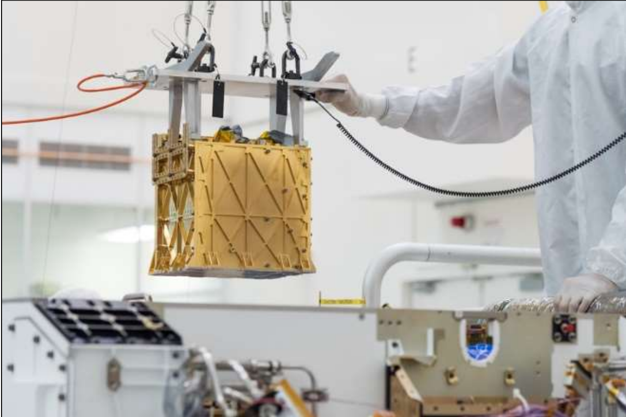
Technicians at NASA's Jet Propulsion Laboratory, in Pasadena, California, lower MOXIE into the body of the Perseverance rover prior to launch Credit: NASA/JPL-Caltech
