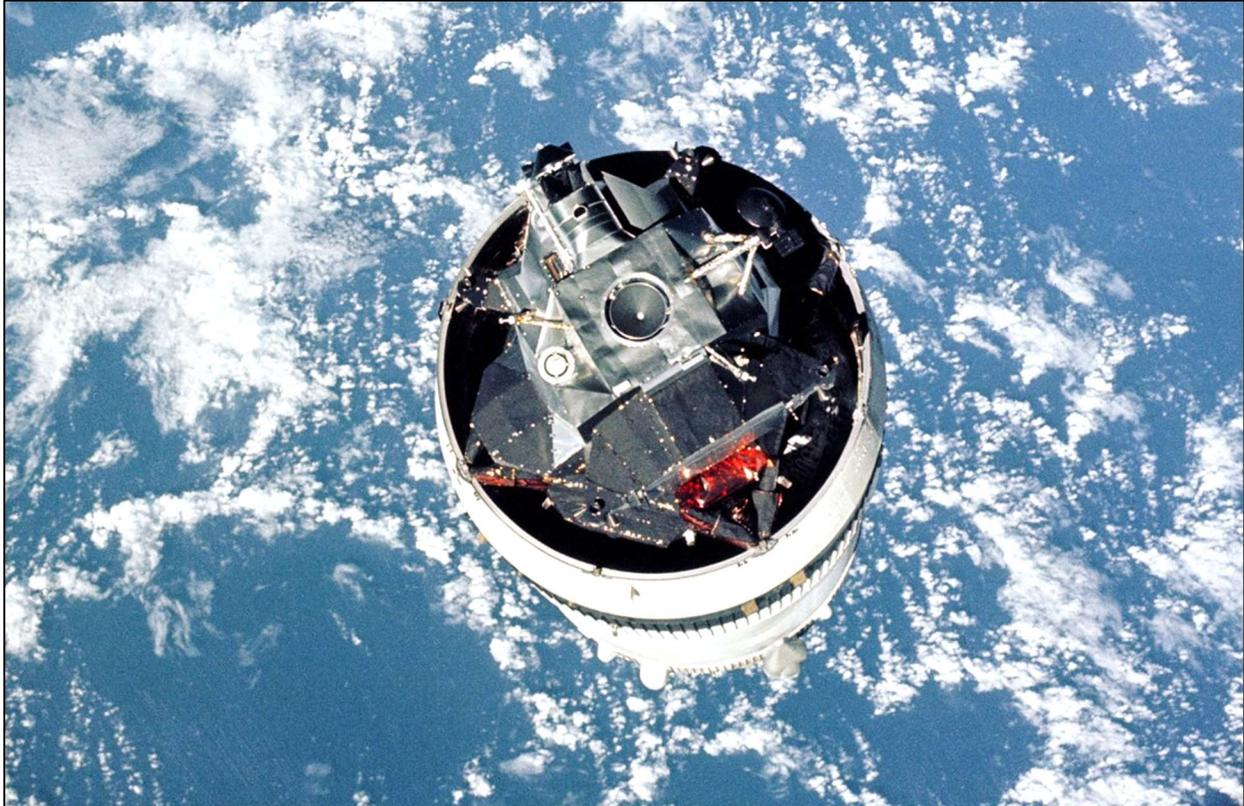
The Apollo 9 LM, nicknamed 'Spider,' shown in its launch position atop the Saturn V S-IVB third stage, its legs folded underneath. The image was taken from the CSM, nicknamed 'Gumdrop,' as it turned to face the LM. The conical drogue docking unit is visible at the top of the LM.
