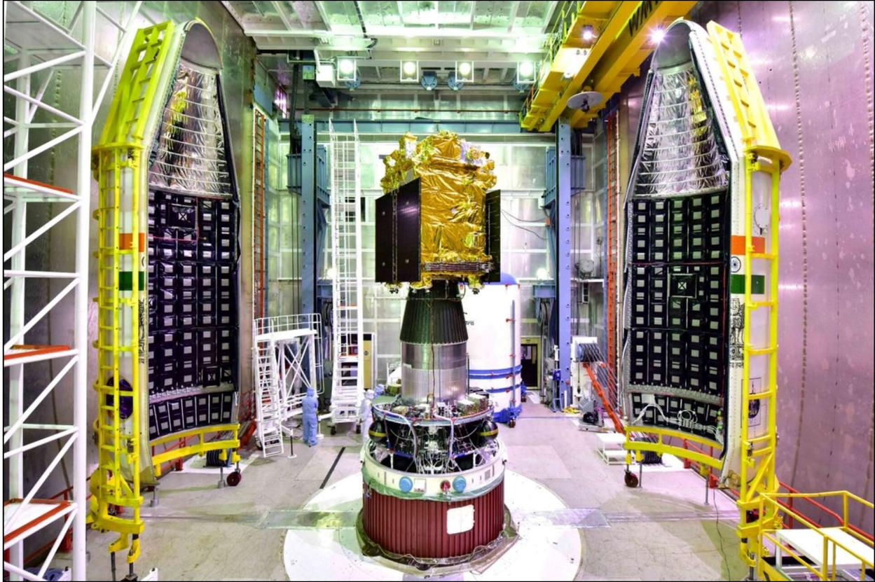
Aditya-L1 atop PSLV C57's fourth stage, shortly before being enclosed in the payload fairing. (Credit: ISRO)
