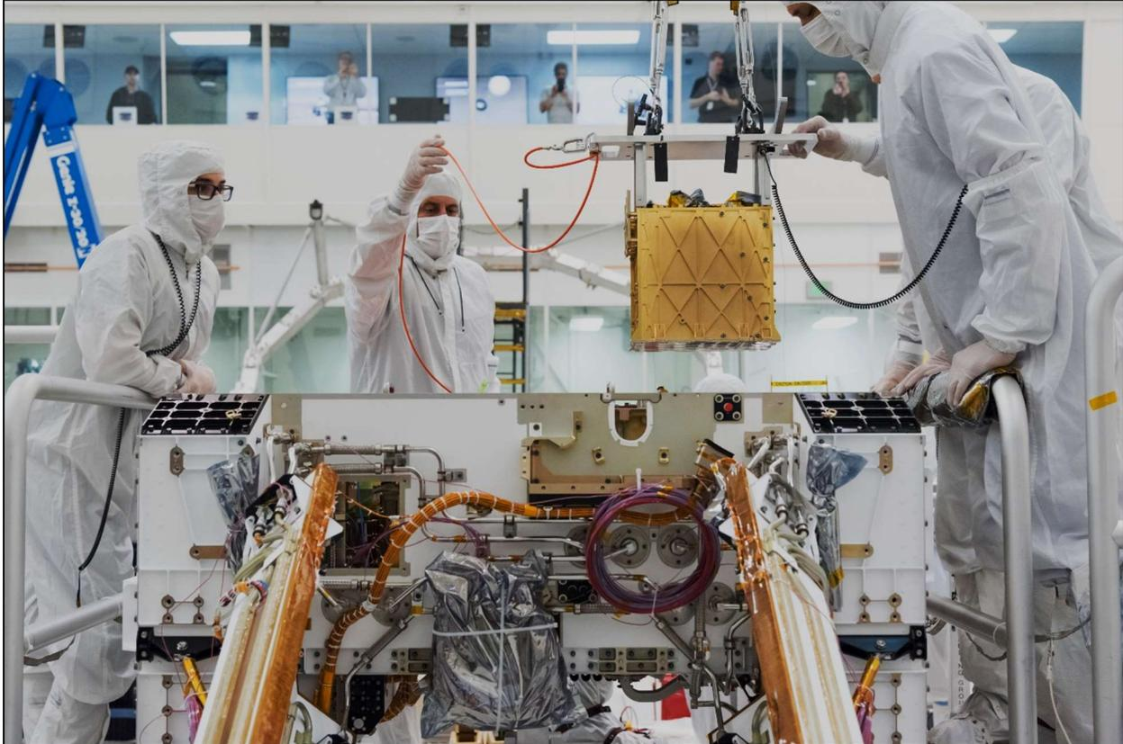
MOXIE, contained within the gold-colored package, being installed into the chassis of the Mars Perseverance rover at NASA's Jet Propulsion Laboratory, in Pasadena, California
