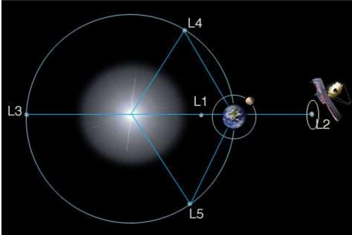
Five locations discovered by mathematician Joseph Lagrange where the gravitational forces of the Sun and Earth (or other large body) and the orbital motion of the spacecraft are balanced, allowing the spacecraft to hover or orbit around the point with minimal expenditure of energy. The L2 point (location of the Euclid and James Webb telescope) is situated 1.5 million kilometers beyond the Earth (as viewed from the Sun).
