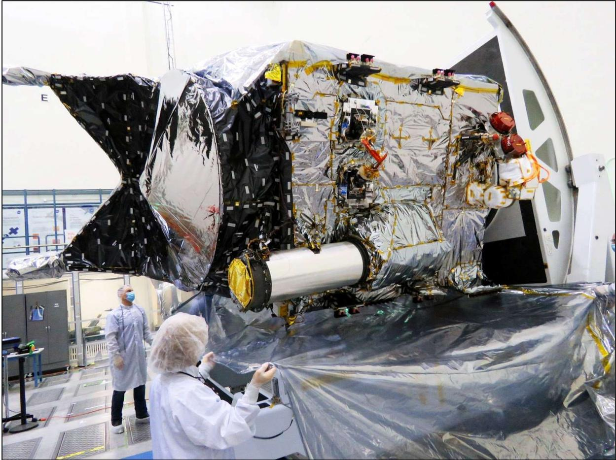
The DSOC flight laser transceiver, distinguished by its prominent tubular sunshade, is mounted on the side of the Psyche spacecraft. The photo was taken during launch preparations.
