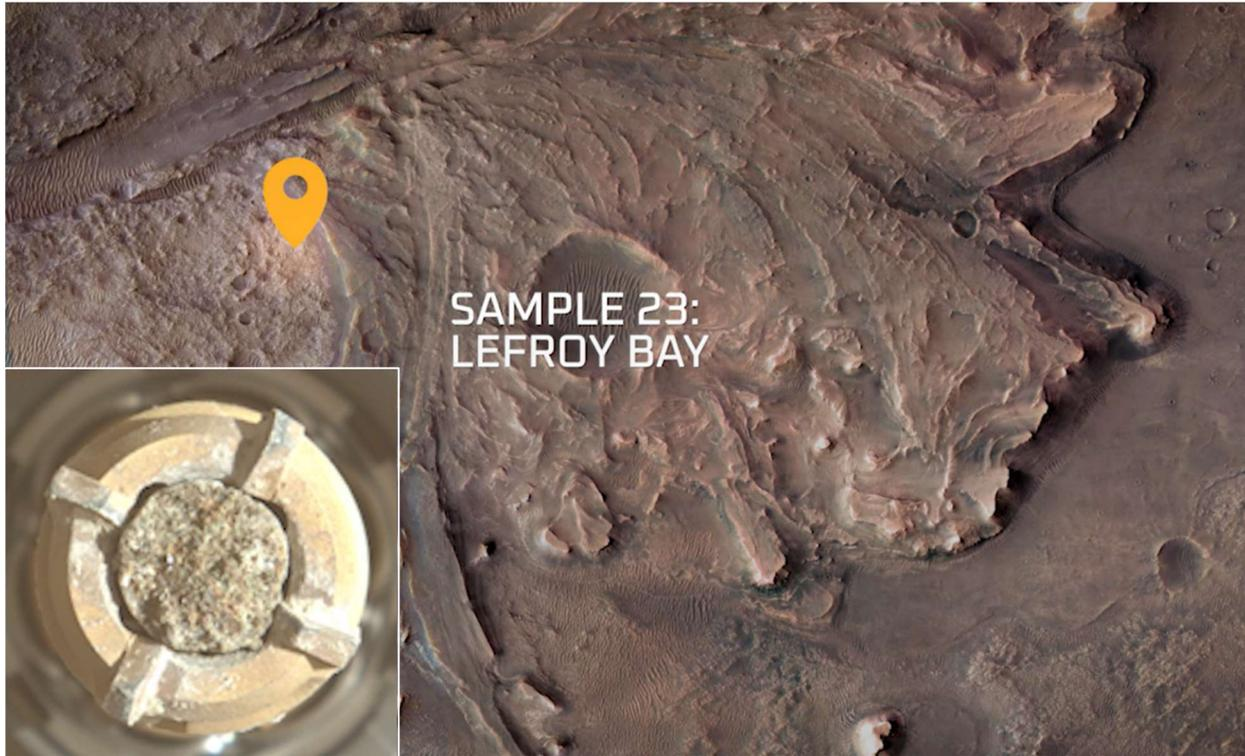
Insert: Core sample No. 23 after being extracted by the rover's rock drill and prior to being transferred into a sample storage tube - imaged by the rover's Left Mastcam-Z camera.
