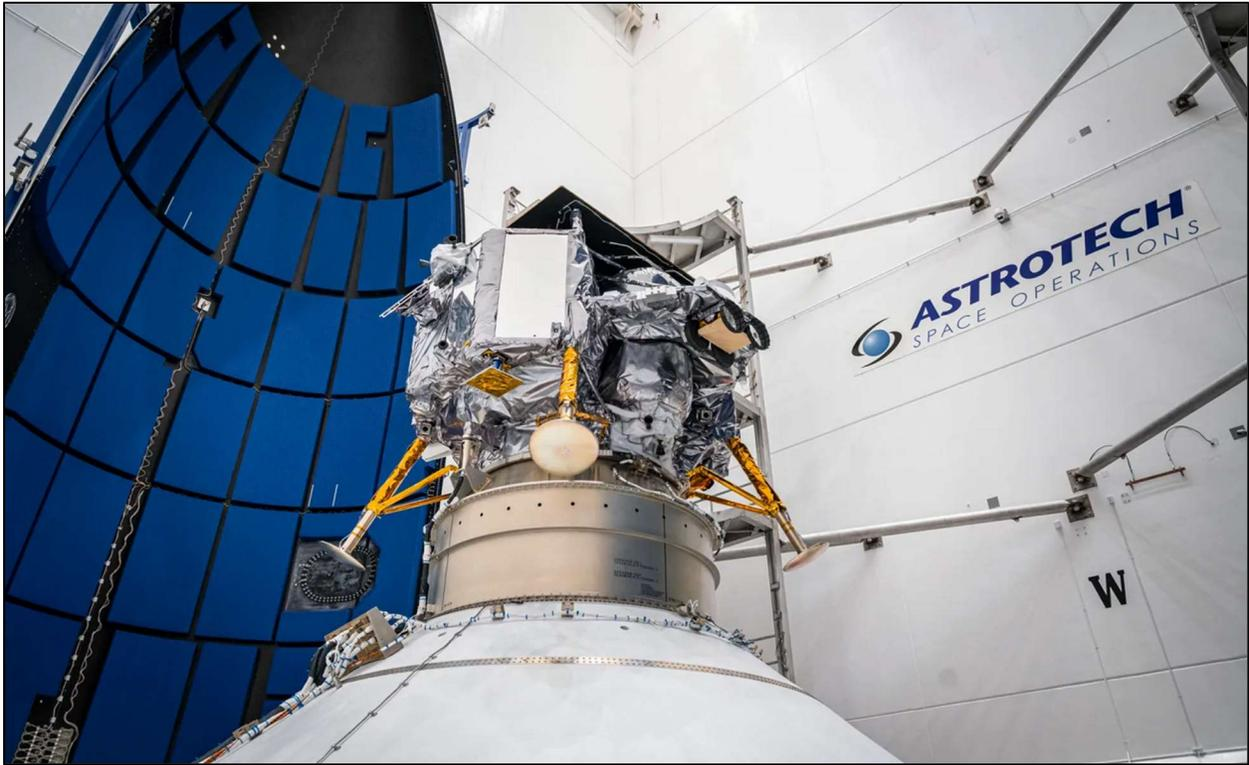
Pre-launch photo of Astrobotic's Peregrine lunar lander prior to being encased within the payload fairings (nose cone) of ULA's Vulcan rocket
