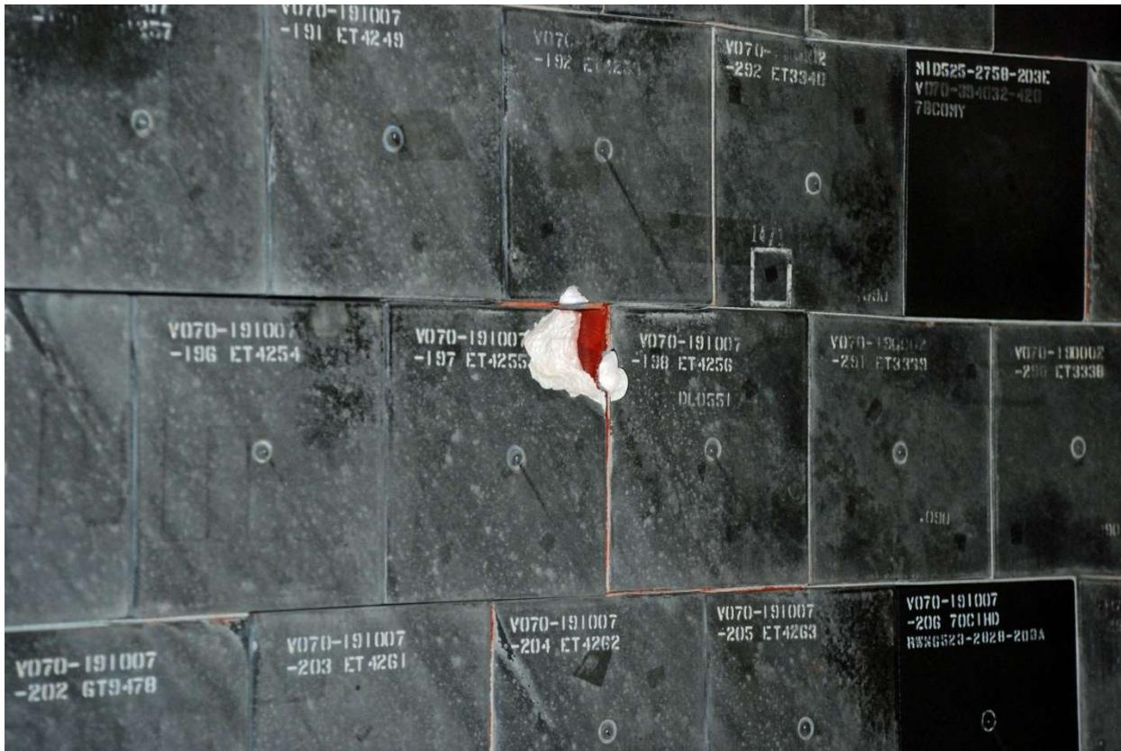
Closeup view of the black HRSI (high-temperature reusable surface insulation) tiles that provided passive thermal control in orbit and shielded the shuttle from the searing heat of re-entry when temperatures reached 1,200 -2,300°F (650 - 1,260°C). Damage incurred during its last flight is also visible in a number of the 23,000 HRSI tiles on the vehicle.
