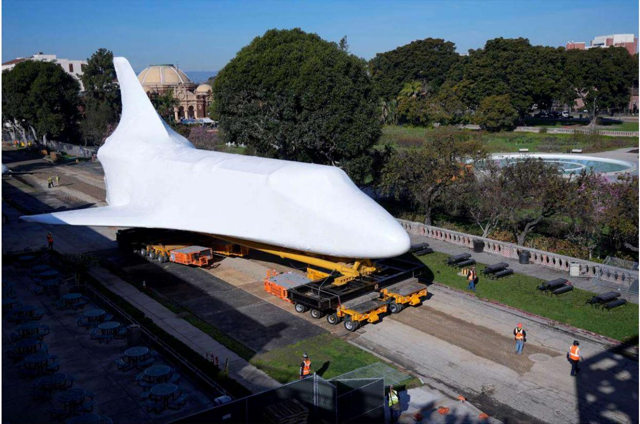
Shrink-wrapped shuttle Endeavour being moved and lifted into the Samuel Oschin Air and Space Center, completing the “stack”
