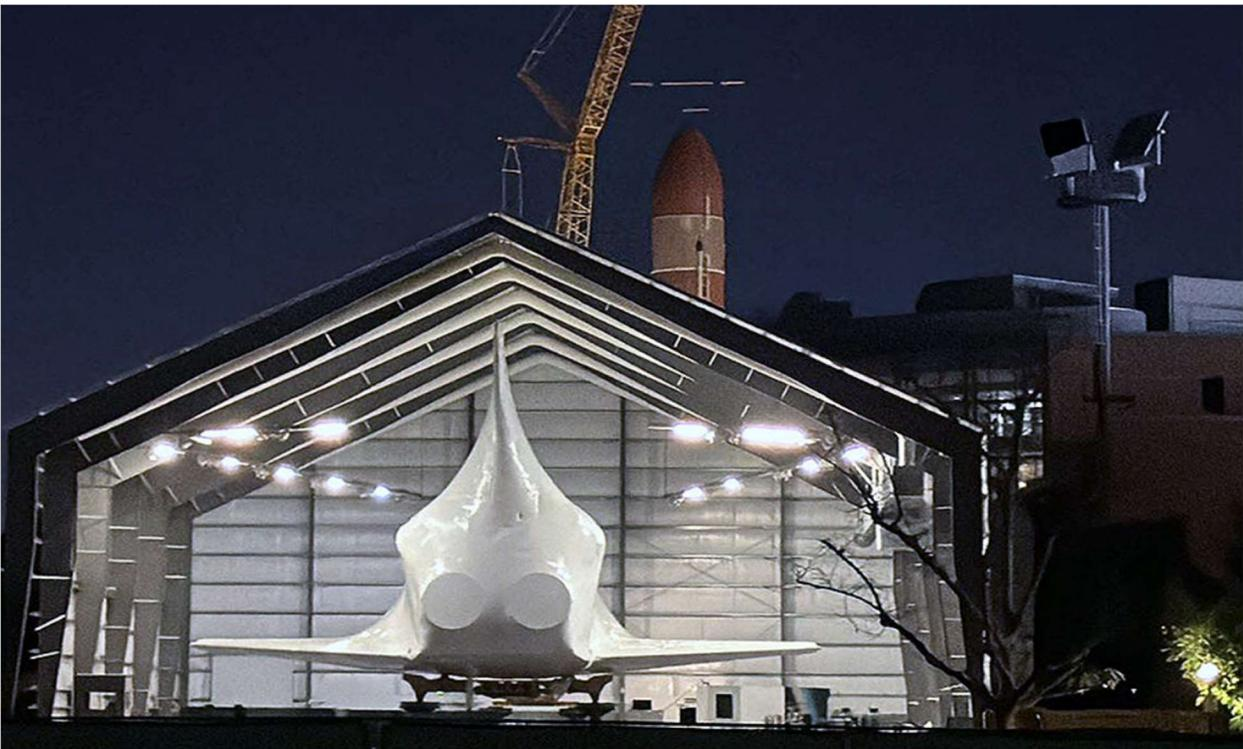
Space shuttle Endeavour, covered in shrink wrap, waits to be lifted and stacked while the crane moves the External Tank in the background.
