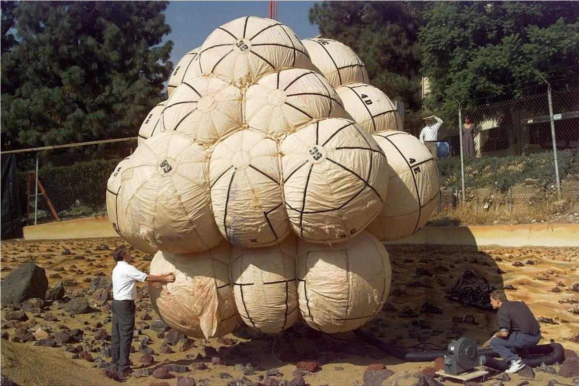
The landing of the Mars Exploration Rovers was cushioned with a cluster of double-bladder airbags (with the rover cradled inside) which were released about 40 - 60 feet (15 - 20 meters) above the surface.
