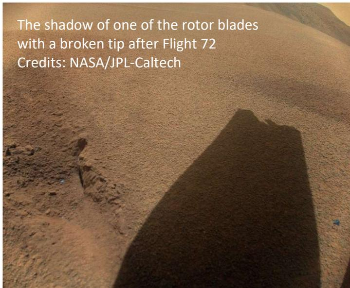
The shadow of one of the rotor blades with a broken tip after Flight 72
