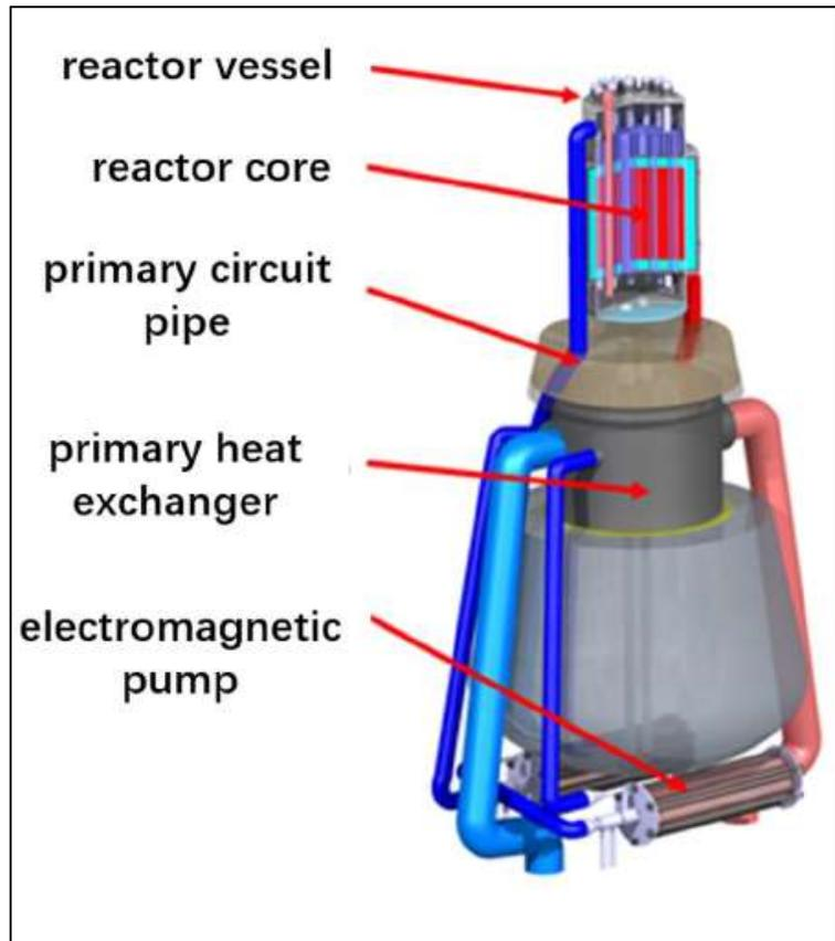
Schematic diagram of the ultra-small lithium-cooled space nuclear reactor (Song et al., 2021)
