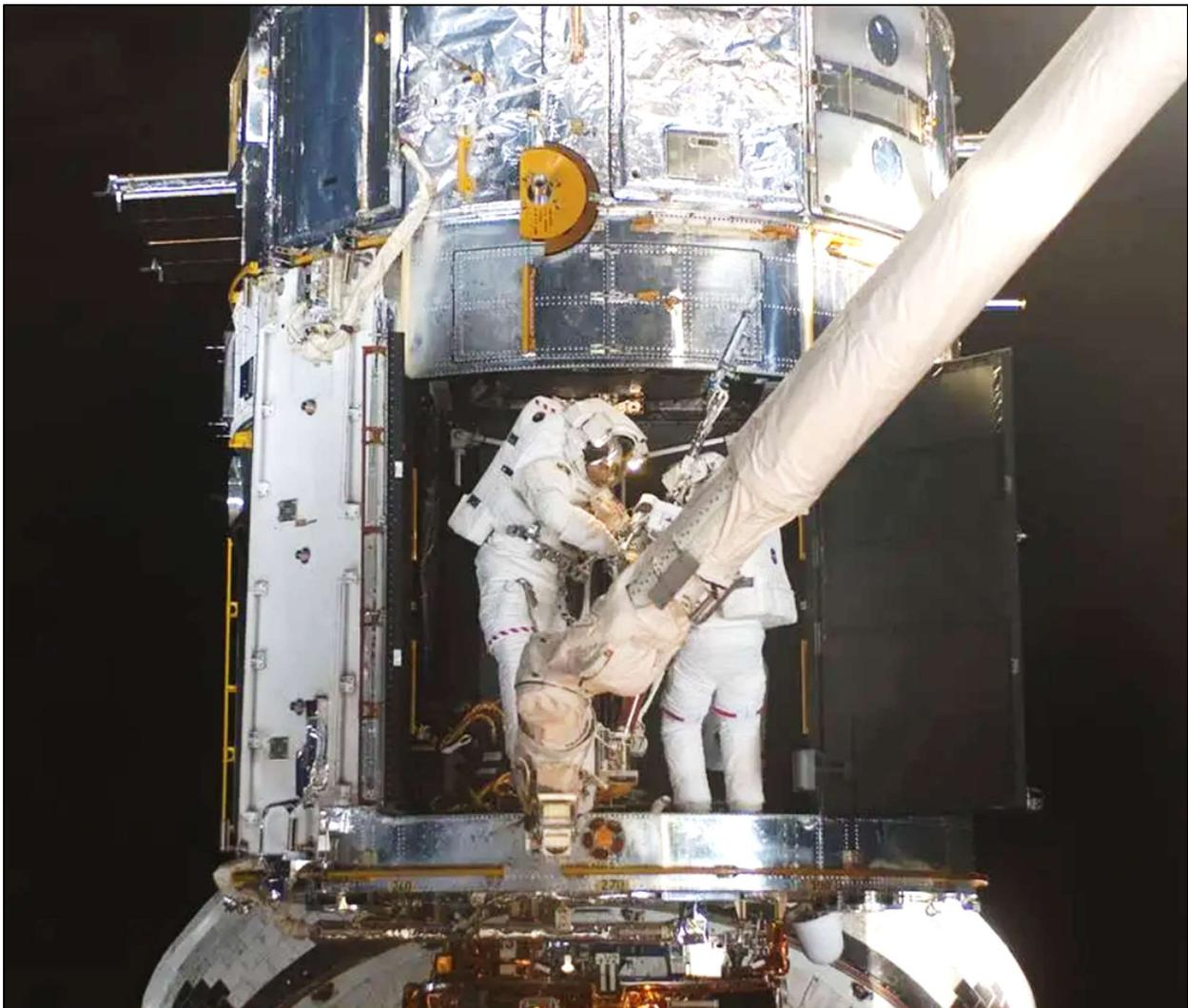
Mission Specialists Michael Good (left) and Mike Massimino continued repairs and improvements to the Space Telescope Imaging Spectrograph during the mission's fourth spacewalk while the telescope is parked in the shuttle's cargo bay.
