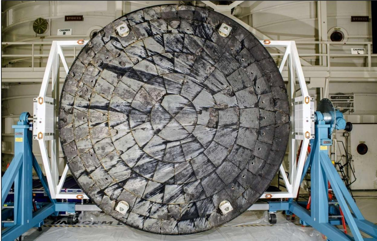
The thermal shield from NASA's Orion spacecraft. The 16.5 feet in diameter (5 meters) shield was removed from the spacecraft at the conclusion of the Artemis I test flight for inspection. Credit: NASA
