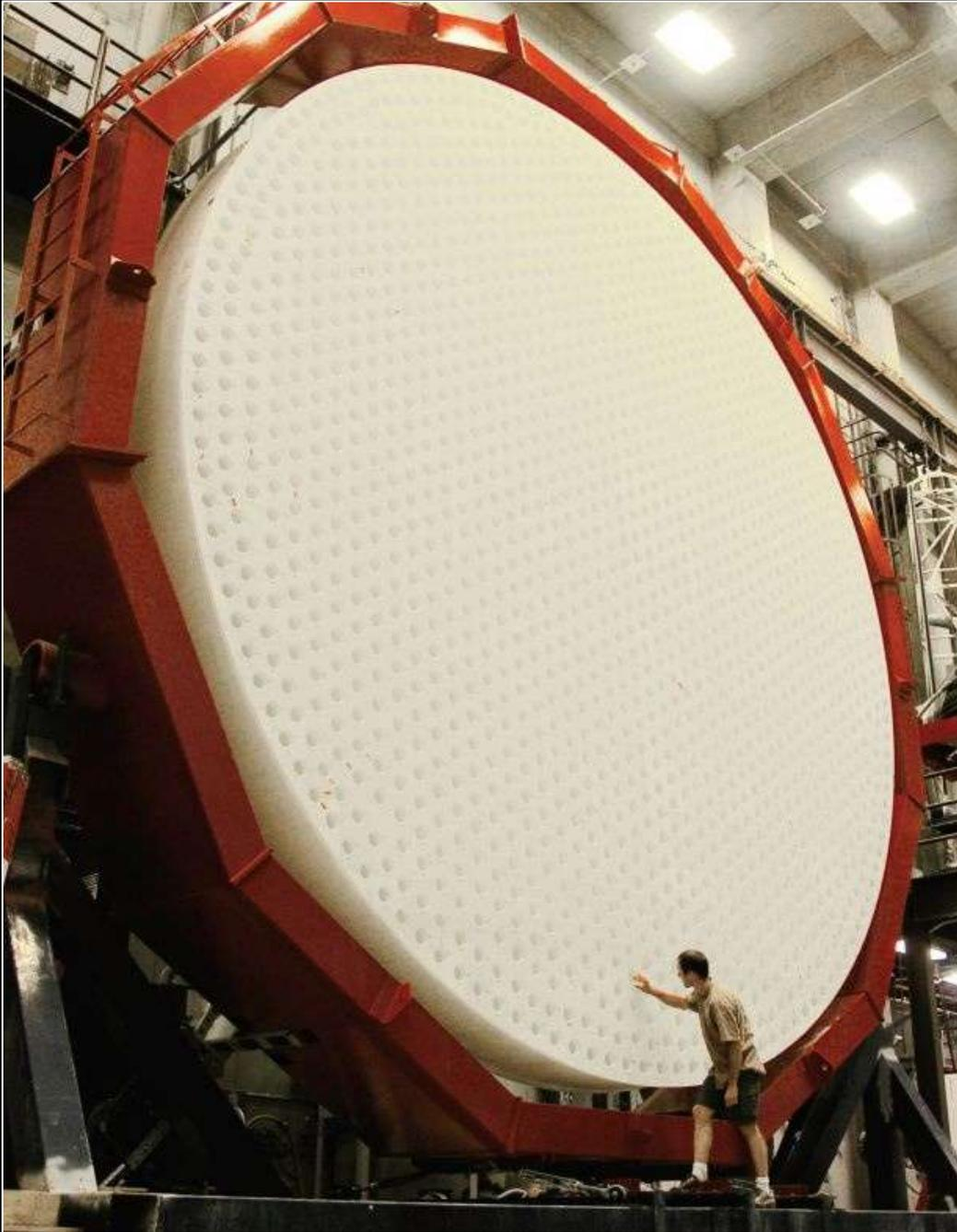
The back surface of one of the seven mirrors cast for the Giant Magellan Telescope. Each 8.4 meter (27.5 foot) mirror is formed from nearly 20 tons of pure optical glass in a rotating furnace at the University of Arizona's Richard F. Caris Mirror Lab located beneath the football stadium.
